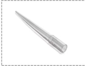
Mostly used in research work for transferring small volume of liquids with high precision
